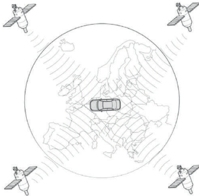
Figure 3.157 Four satellites determine vehicle position more accurately
